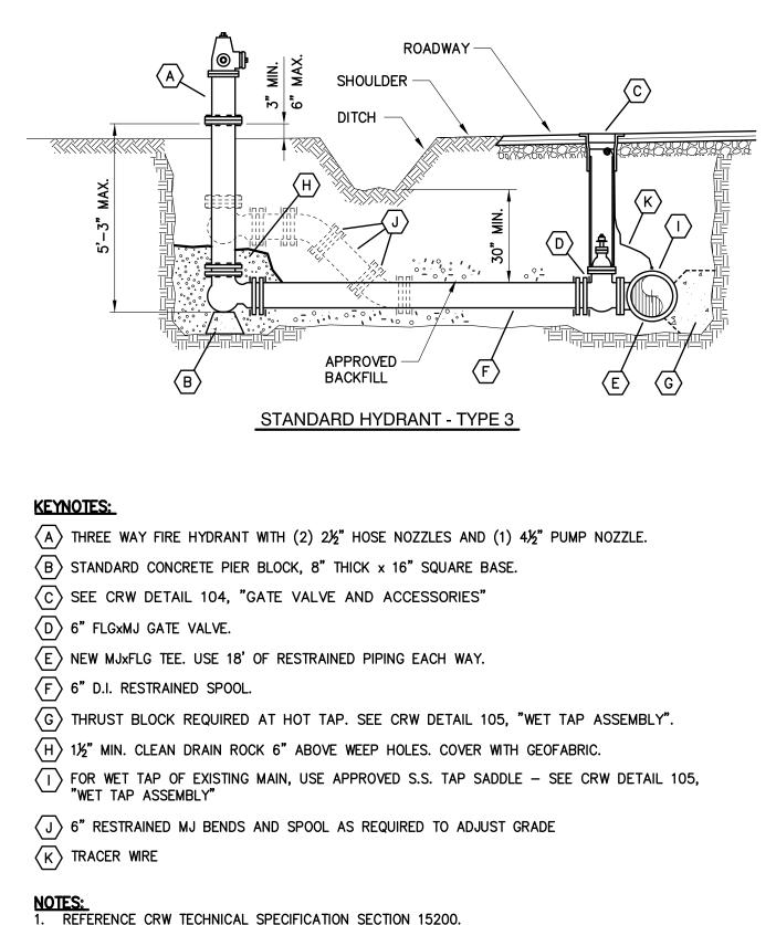
INSTALL MJ BENDS AS REQUIRED TO ADJUST GRADE TO COMPLY WITH MAXIMUM FIRE HYDRANT BURY REQUIREMENTS.
