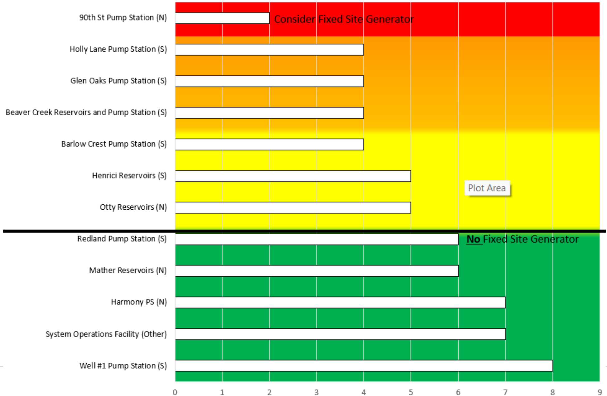
Generator Study Score (Low Number = Needs Generator)
